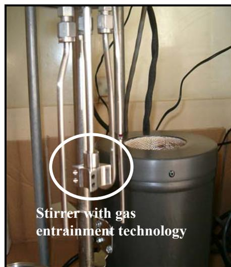
*Gas enters openings near the top of the shaft and is expelled through dispersion ports located at the tips of the impellers. As with all impellers, the speed of the stirrer (800 – 1200 rpm) creates a vacuum at the tip of the impeller. In this system with dispersion ports located at the very tips of the impellers, the higher the stirring speed - the higher the vacuum - and the higher the driving force for this very effective gas dispersion system.*
