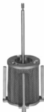
*The catalyst is loaded in a basket to protect it from grinding during operation. The specially designed stirrer combines radial flow and gas entrainment technology to provide an improved mixed gas and liquid flow through the catalyst bed. Thus, the three-phase mixing produced is comparable to the conditions in a fixed-bed reactor and allows an easy screening of the catalysts.*
